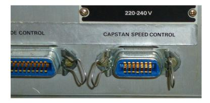
The standard version of the **A80 Quartz-Control** is ready for use with the A80 in the speed version 7 1/2/15 ips (19/38 cm/s).
