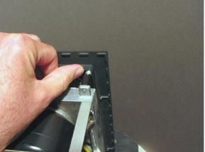
upper fixing points consist of 3 positive locking sockets
