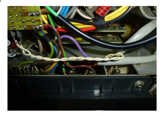
Pull the white cables from the supply PCB and push it onto the flatconnectors on the Mute PCB.
