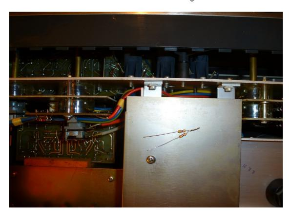
installed first solder the common side on the GND solder lug
