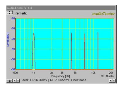
The frequency spectrum looks as depicted if the adjustment is correct. The tape deck is switched to "mono" !
