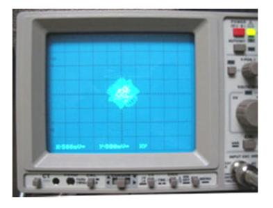
In this screenshot Lissajou's figure is shown if the playback head is accidently to a false maximum. With this tape it is easy to calibrate the playback head to it's main correct position without mistake.
