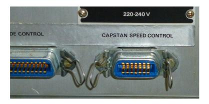
The standard version of the **A80 Quartz-Control** is ready for use with the A80s in the speed version 7 1/2/ 15 ips (19 / 38 cm/s).
