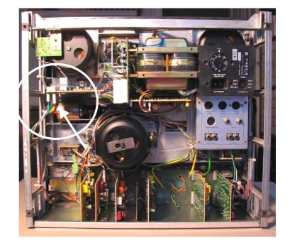
This connector is to be pulled out
