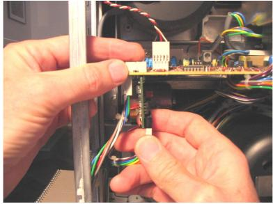
Plug in B77 Pause Memory using the other hand for counter-pressure
