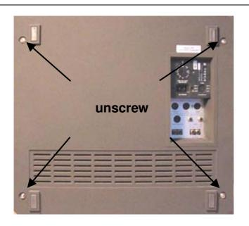
Unscrew the four phillips screws on the backside of the B77 case:
