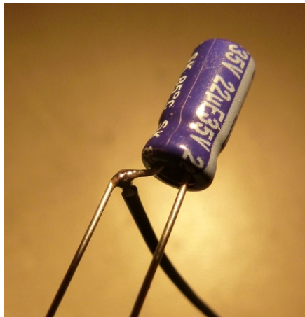
detail of wire soldered to the 22uF cap.
