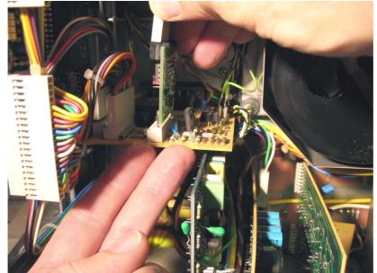
Plug in PR99 Pause Memory using the other hand for counter-pressure
