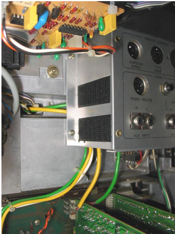
Position of the hooked velcro strips for mounting the Quartz-Control
