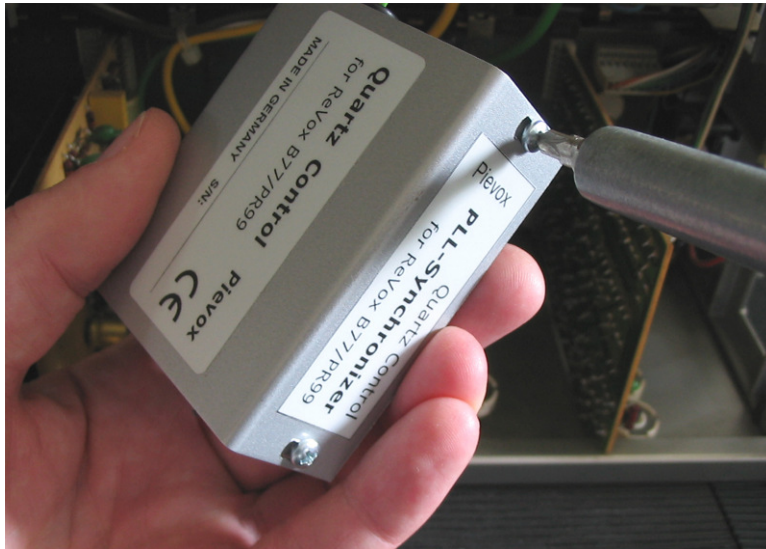
unscrewing the Quartz-Control
