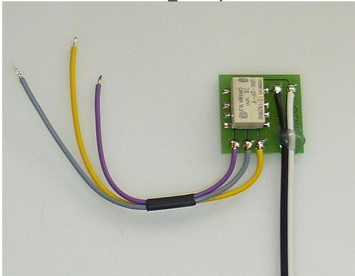
A77-D\_MMR PCB Installed on the Dolby connection board 3 solder joints
