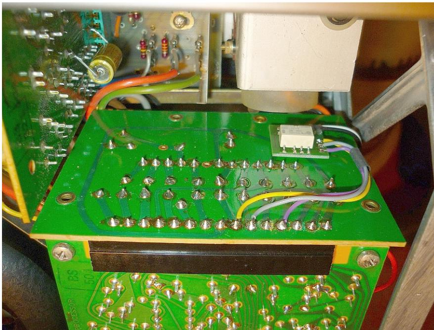
Connections on the Dolby Connection PCB from right = pin1
